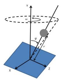
Figure 1: Heavy ball sliding on a rotating wire
