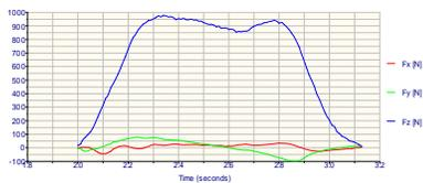
Fig.11. *Forces diagrams for the start with the left foot*
