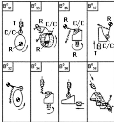
Fig. 1. Elementary cam mechanisms[9]
