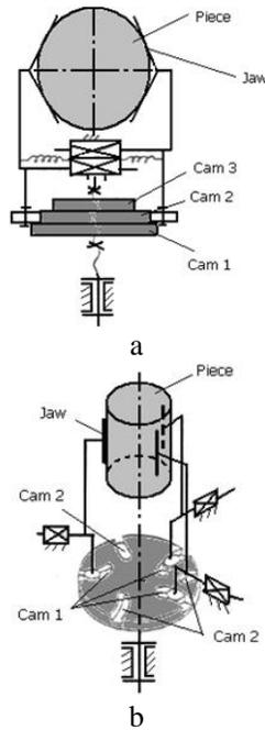
Fig. 3. Structural schemes with multiple cam[15]
