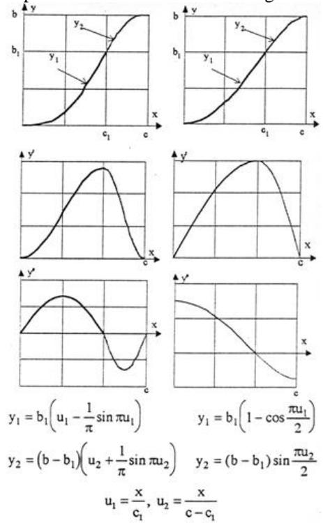
Fig. 6. Compound kinematical functions [14]
