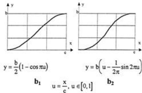
Fig. 5. Simple kinematical functions [14]
