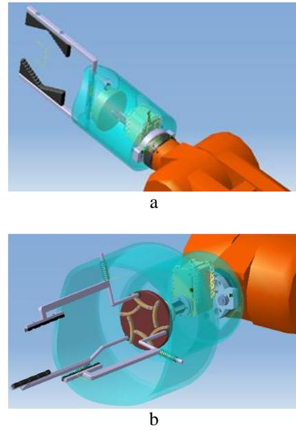
Fig. 7. Gripping mechanisms with cam: CAD models
