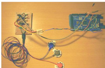
Fig. 3. *Electrodes connected to the amplifier and this one to Arduino Mega 2560 board.*
