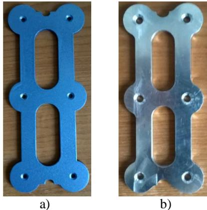
Fig. 4. The cervical plates PCP-01-F obtained by: water jet cutting (a), and classical fabrication (b).
