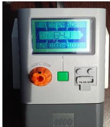
Fig.12 *Recording data with Energy Meter*
