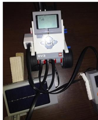
Fig.13 *Display of the angles measured by the gyro sensor*
