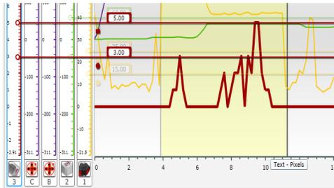
Fig.1 *Graph programming for colour, gyro and ultrasonic sensors*
