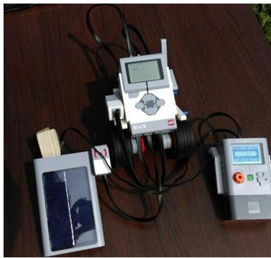
Fig. 7. *Stand for measuring the captured energy using the solar panel*
