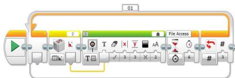
Fig. 8 *Program for measuring angles with the gyro sensor*
