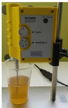
Fig. 1. Ultrasonic Processor UP100H during epoxy treatment [2]
