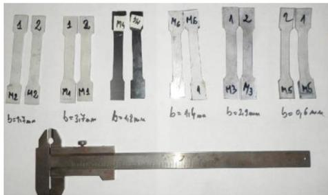
Fig. 5. Test specimens made of the plastic materials
