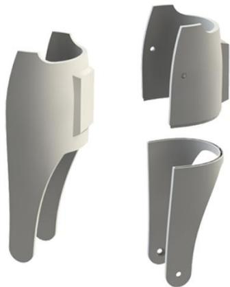
Fig.3. CAD model of the upper part of orthosis
