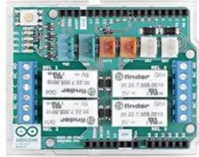
Fig.8. *Module with 4 relays [11]*
