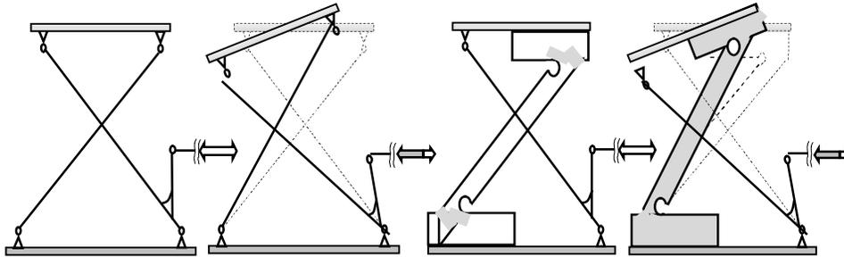
Fig.8. Four bar linkage
