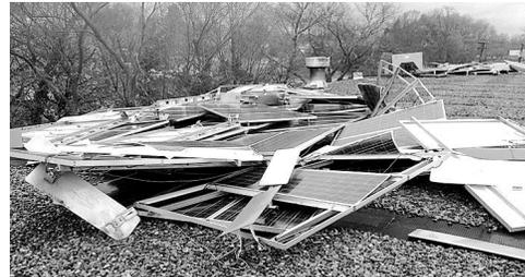
Fig.1. *Important solar panel damages caused by wind*
