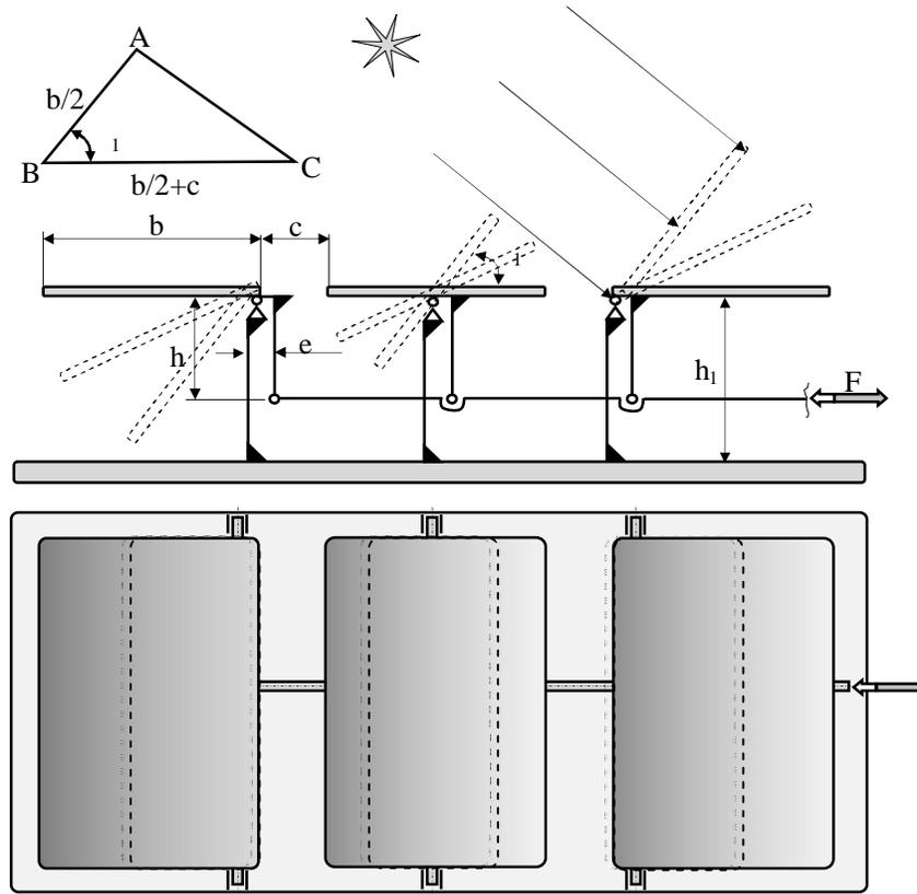
Fig.5. Frame with three asymmetrical panel axes
