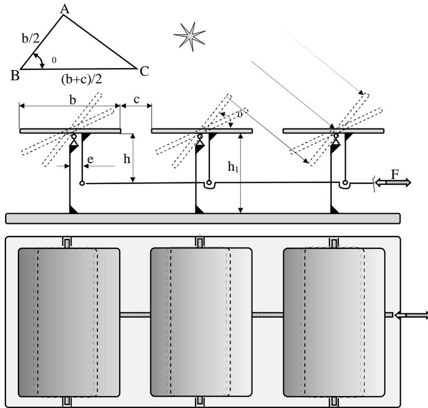
Fig.4. *Frame with three symmetrical panel axes*
