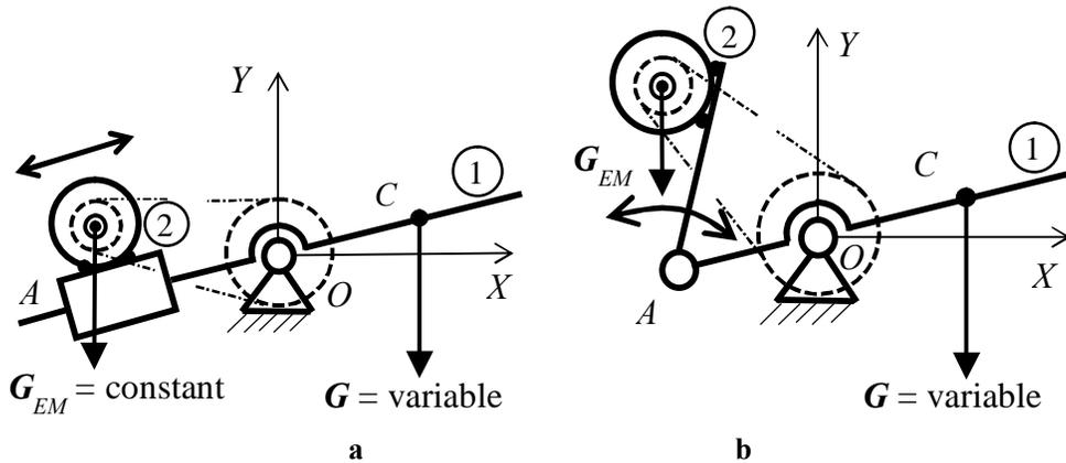
Fig. 2. Replacing the fixed position of the counterweight (electric motor) by a movable one
