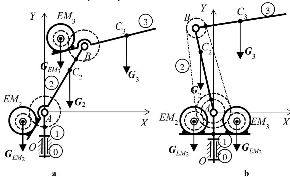
Fig. 1. Internal mass redistribution in the case of robot manipulator by using electric motors as counterweights
