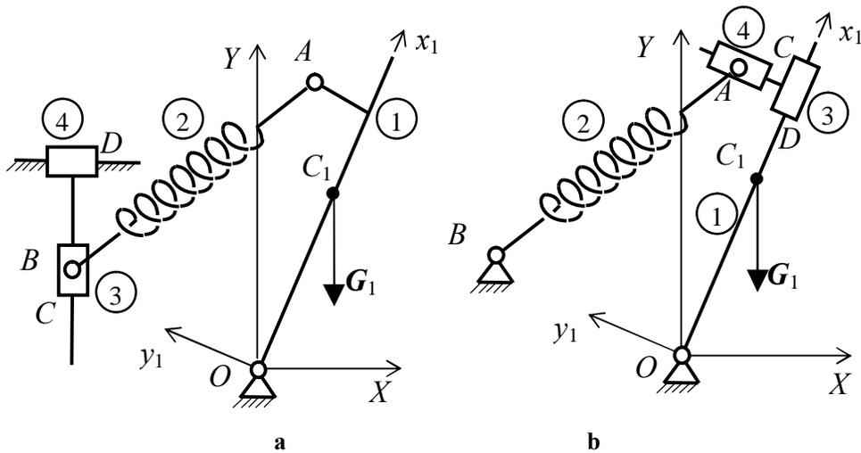
Fig. 3. Replacing the articulation points of helical spring by movable ones
