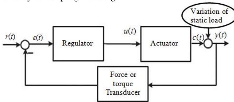
Fig. 4. Controller scheme
