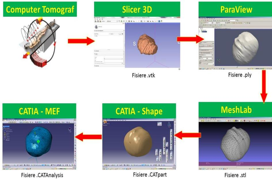
Fig. 8. *The methodology for the analysis using MEF*
