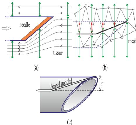
Fig. 7. (a) The progress of the bevelled needle tip inside tissue; (b) mesh nodes sliding in 2D along a unidimensional tip-bevel model; and (c) tip bevel model in 3D [2]
