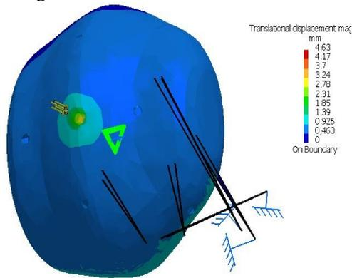
Fig. 11. Analysis of deformations and displacements occurred when inserting the needle
