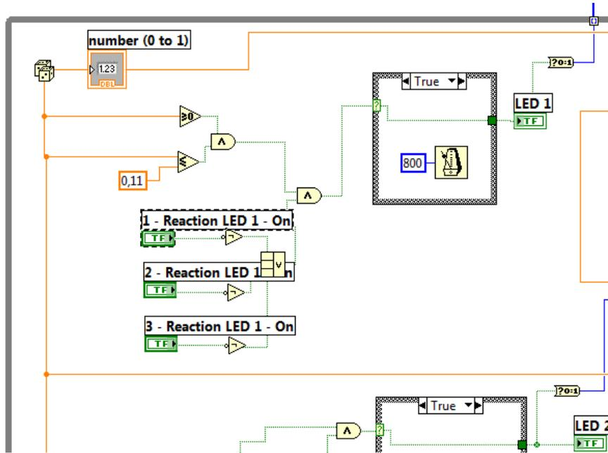
Fig. 5. The While-Loop main programming structure for continuously testing running
