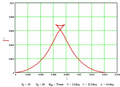
Fig. 5. The influence of the taper angle of the rollers,  $\beta$  on the form of teeth profile
