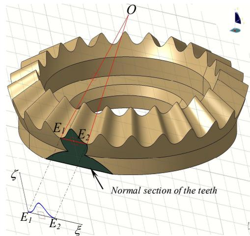
Fig. 6. 3D model of the whole gear
