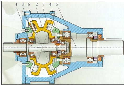
Fig. 1. Diagram of the planetary precessional transmission
