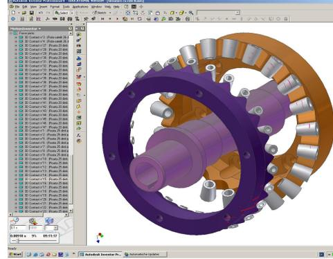
Fig. 2. Computerized model of the planetary precessional gear
